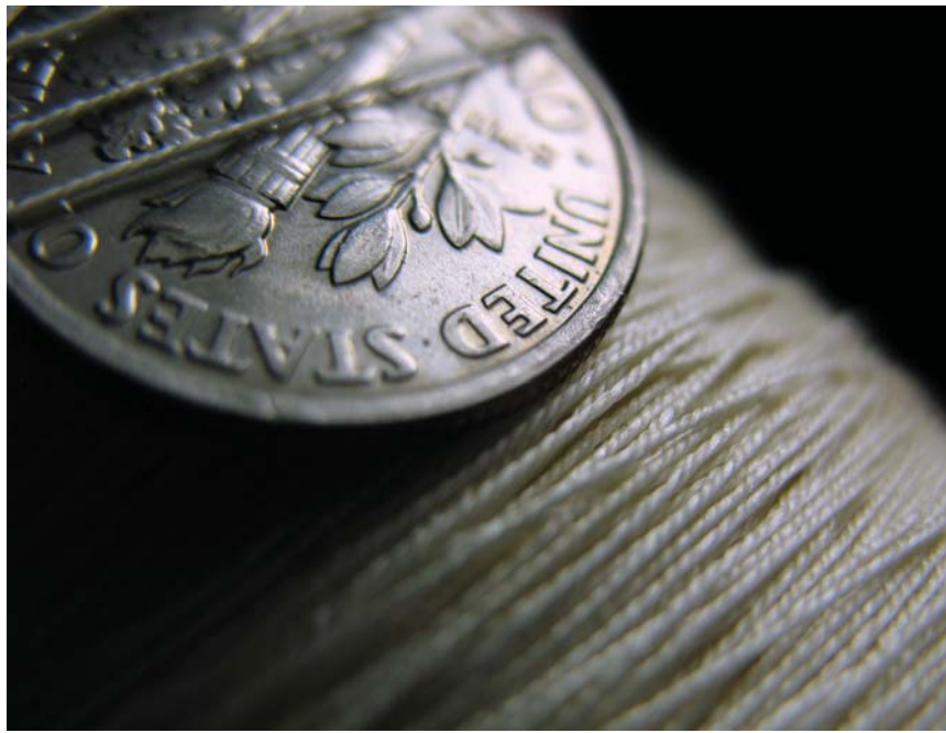
Michael Cook's handmade three-ply organzine before degumming is stiff and waxy. A U.S. dime is shown for scale.
