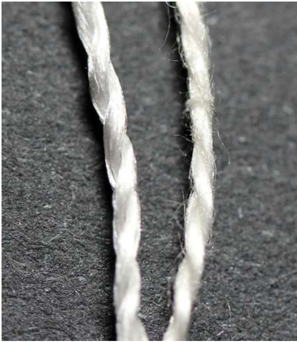
A reeled strand at left and a spun strand at right.
