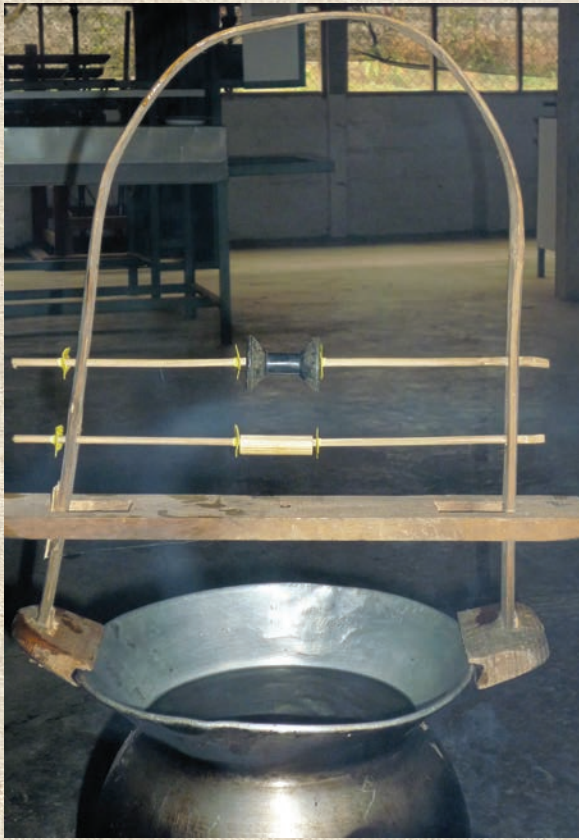
Above: The filaments from a number of cocoons are threaded through the reel. Left: A traditional Lao silk-reeling set up.
