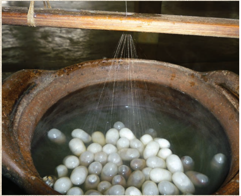
Above: The filaments from a number of cocoons are threaded through the reel. Left: A traditional Lao silk-reeling set up.
