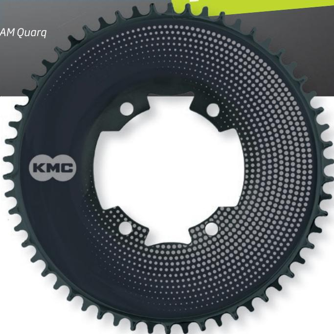
KMC introduces a new chainring series for time trial and triathlon - tested and approved by Pro Teams. Precision CNC-machined from high-strength AL7075-T6 aluminum, these chainrings deliver maximum stability, efficiency, and aerodynamics. The narrow-wide tooth profile ensures secure chain retention and reduces friction - essential for race performance.
