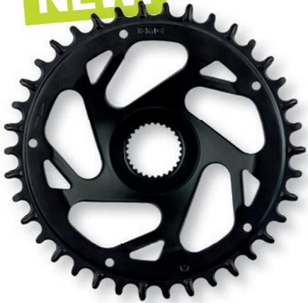
Not compatible with 12-/13-speed flattop chains
