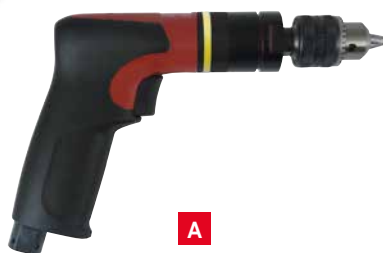
A DR350 Series 350 W (0.5hp) / 550 to 20000 rpm
