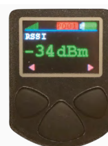
Real-time Wi-Fi signal strength check
