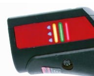
4 color LEDs for tightening / tool status
