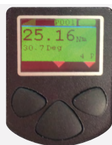
Tightening result on the OLED display
