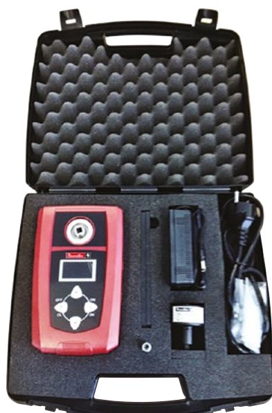
■ Embedded Transducer & Battery
