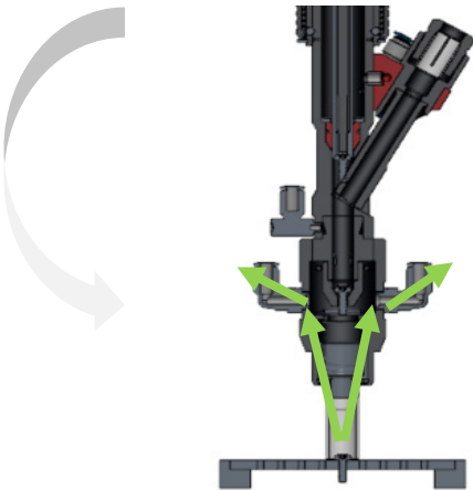
Step 3: Once tightening is complete, a vacuum system removes any dust generated during the process
