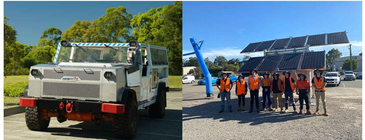
DRIFTEX is the first battery operated vehicle to operate in an intrinsically safe environment
