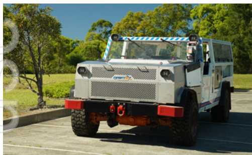
DRIFTEX – the first battery operated vehicle to operate in an intrinsically safe environment.
