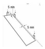
1. Start with a first, full length plank (n°1), which comes in the top left corner of your room. Preferably lay the 2 sides with tongue towards the walls and make sure that the expansion joint of 5 mm is
