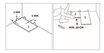
Now take a second tile and cut it to a minimum of 1/3 and a maximum of 2/3 of a panel length as a starting tile ( $n^2$ ) for the second row.
