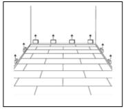
1. For the installation of the last row, you will have to saw the boards lengthwise. You can use a metal striking bar to insert the boards into the click system of the previous row. Please note: hitting the boards too hard or too unevenly can damage the boards and their click connections.
