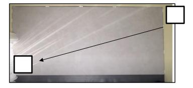
A leftover peace of tile can serve as the starting piece for a new row. Make sure that the 30 cm distance between the end edges is respected.
