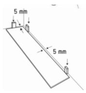
1. Start with a first, full length plank (n°1), which comes in the top left corner of your room. Preferably lay the 2 sides with tongue towards the walls and make sure that the expansion joint of 5 mm is
