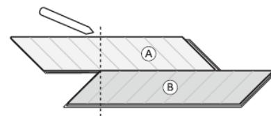
Click the two panels out each other. Take a sharp knife and cut the décor layer of both panels along the line. Make sure that the cutting line is firm and deep enough, otherwise the panel will not break correctly. Replace the cutting blade regularly.
