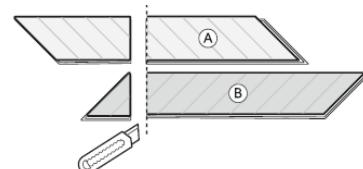
Turn the panels over with the decor side down and sit with your knees on top of the cut line. Make a lever and break the panels in half. The pieces you cut might be used again later at the end of the row.
