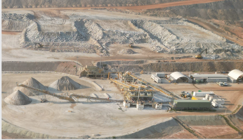
Crushed stockpiles (foreground) and ROM stockpiles (background) December 2023.
