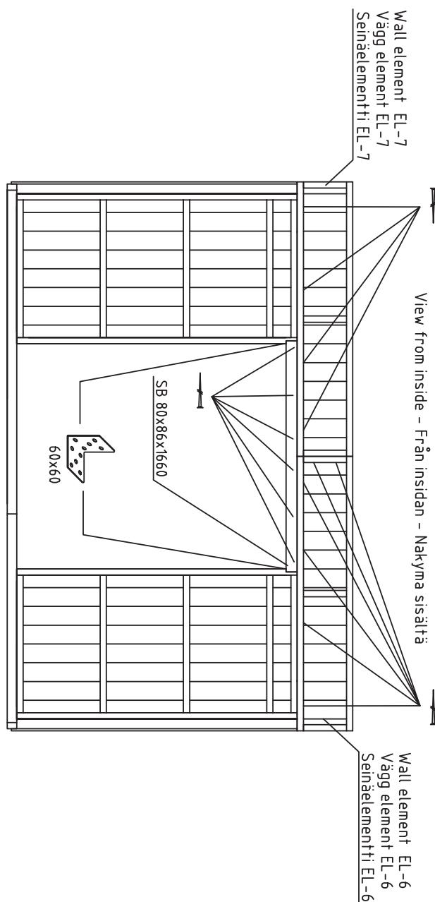
Fix wall element EL-7 with front wall elements with screws 4,5x70 together
