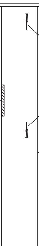
Fix wall element EL-1 with screws
