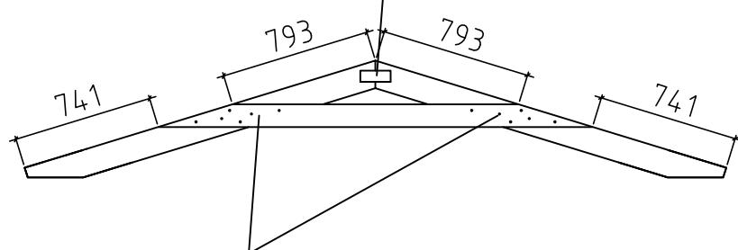
Connect with nails 4x100 (6+6) → on both sides of the ferm
