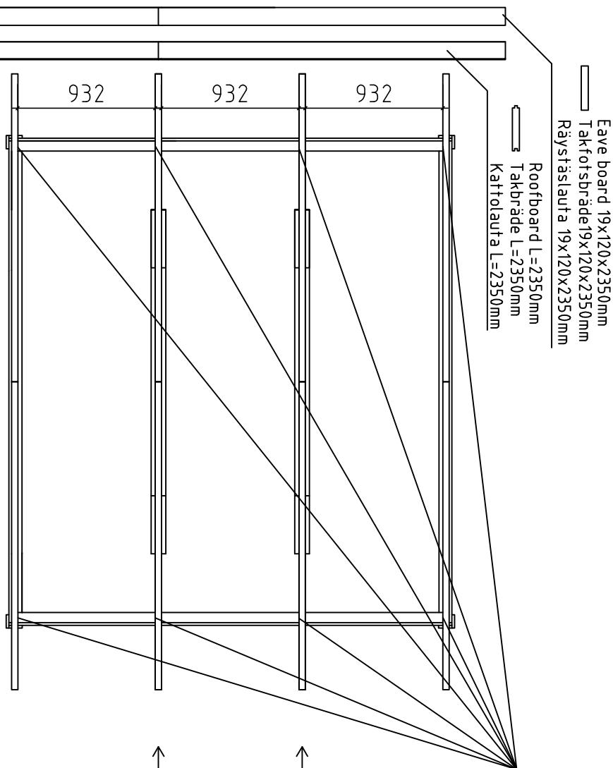
NB!!! max load on the roof 100kg/m<sup>2</sup>
