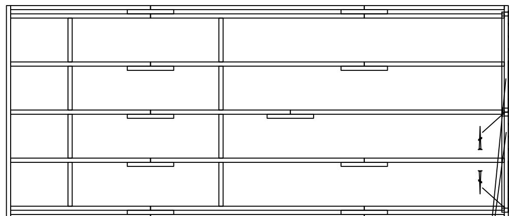
Fix wall element EL-7 with screws 4,5x70 into floorbeam
