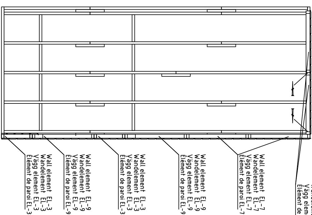
Fix wall elements EL-7, EL-9 and EL-3 with screws 4.5x70 into floorbeam
