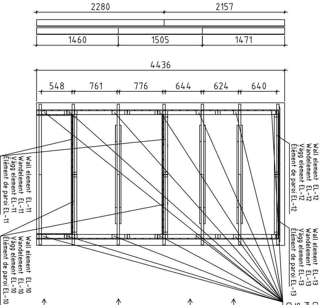
Connect with steel corner 90x90x65+screws 4.5x45 14pcs
