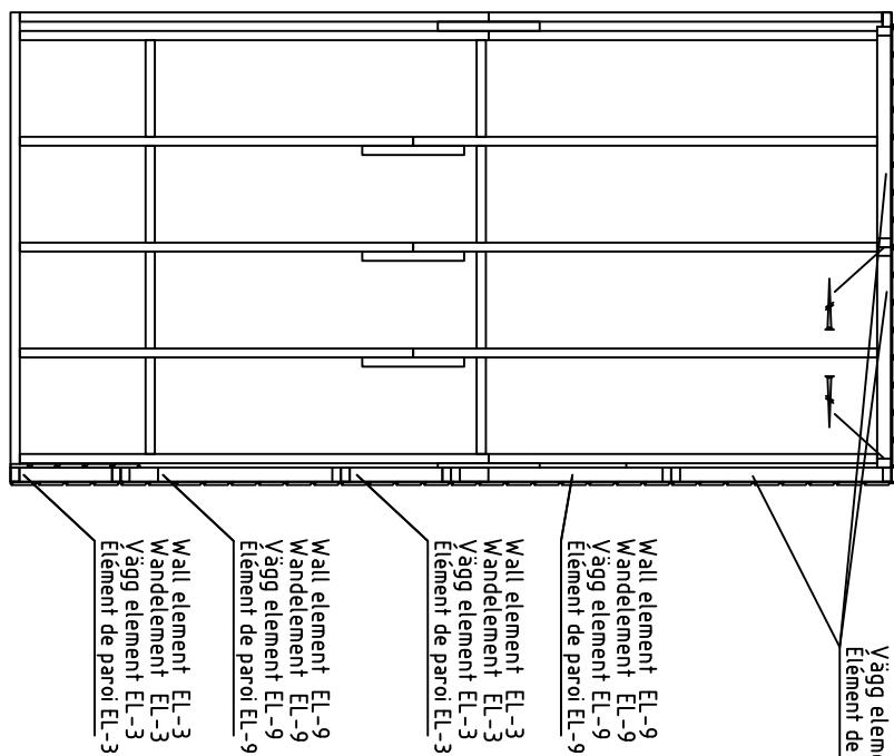
Fix wall elements EL-7, EL-9 and EL-3 with screws 4.5x70 into floorbeam
