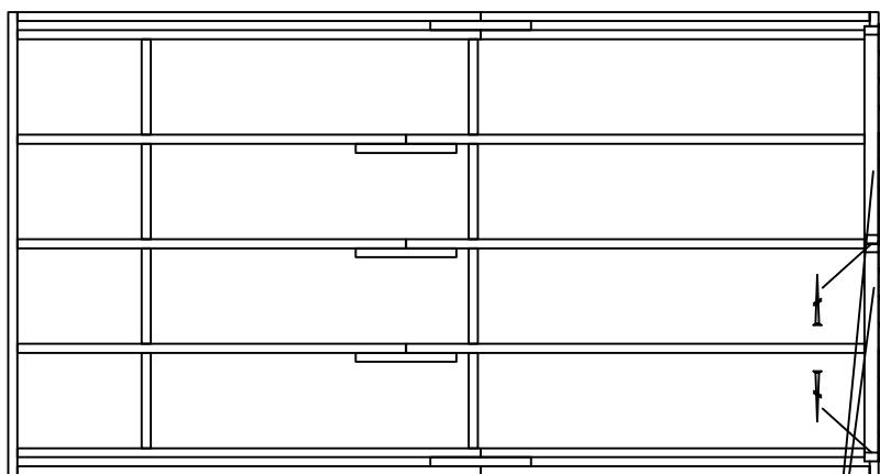
Fix wall element EL-7 with screws 4,5x70 into floorbeam
