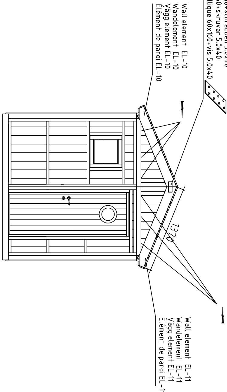
Fix wall element EL-10, EL-11 with back wall elements with screws 5.0x120 together
