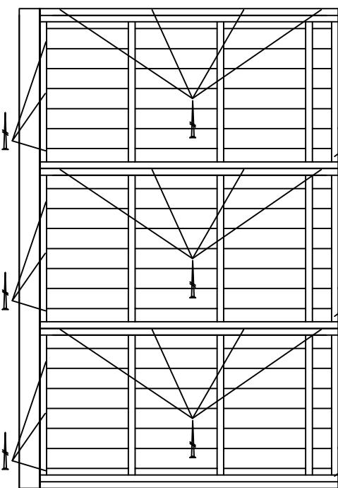
Fix wall element EL-3, EL-1, EL-2 with screws
