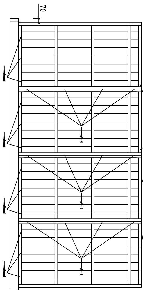
Fix wall element 4xEL-1 with screws
