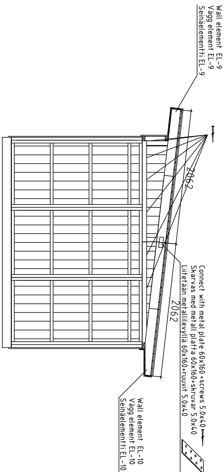
Fix wall element EL-9 with left sidewall elements with screws 5.0x120 together
