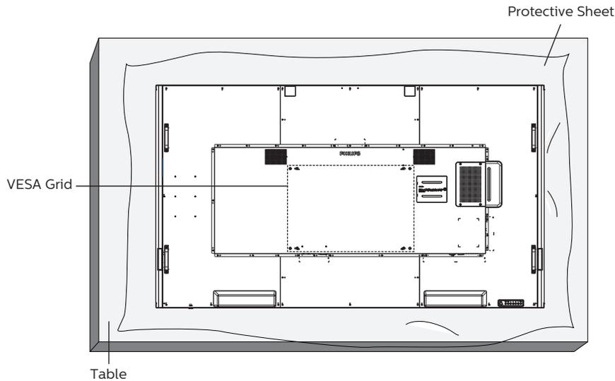
1. Prepare a flat and horizontal surface that is larger than the display and spread a thick protective sheet on it to facilitate your operation without scratching the screen.
