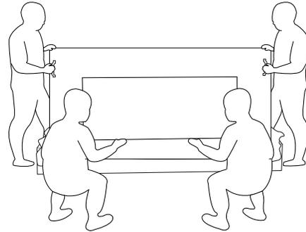
6. Carefully move the display until the bottom handles are out of the box. Two people on the sides should hold the 4 handles, while two others stand at the front and back of the display to support the bottom.
