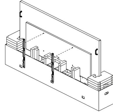
**\* The recommended number of professional personnel for unpacking and installation requirements is at least 2 for 65" & 75" models, and 4 for the 86" model.**
