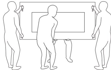
7. The person who was initially at the back of the display should move to the front, so that all four people can mount the display onto the wall.
