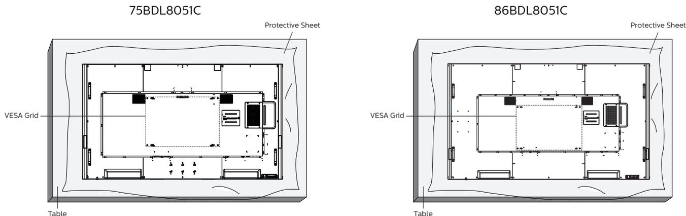
1. Prepare a flat and horizontal surface that is larger than the display and spread a thick protective sheet on it to facilitate your operation without scratching the screen.
