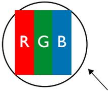
One dot = One Pixel; consists of three sub-pixels of Red, Green, and Blue.
