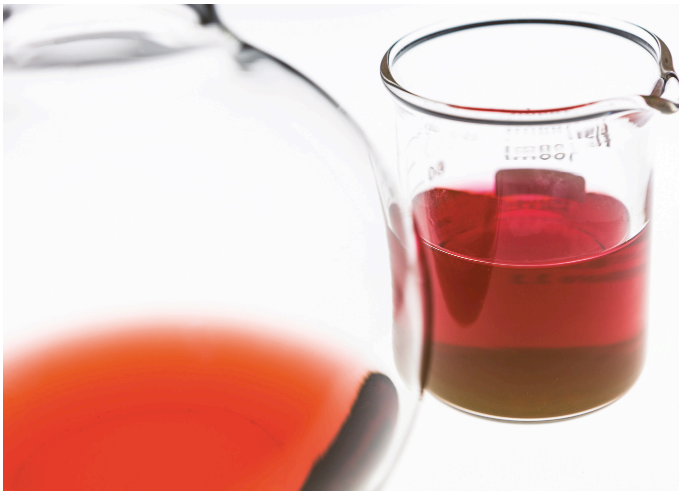
Gold nanoparticles in solution. The distinct colours are a consequence of the tiny metal particles interacting with light. Depending on the size of the particles, the solutions can be blue, purple, red or green. Most LFAs use particles which give a deep red colour. (Photograph copyright World Gold Council)
