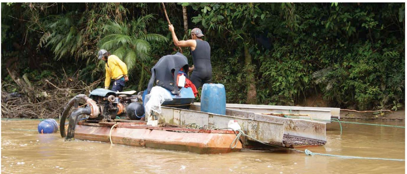
Alluvial miners on the Rio Zarza in south-east Ecuador. A diver guides a suction pump to pull up gravel which then passes over a sluice on the raft. Copyright: Kinross.
