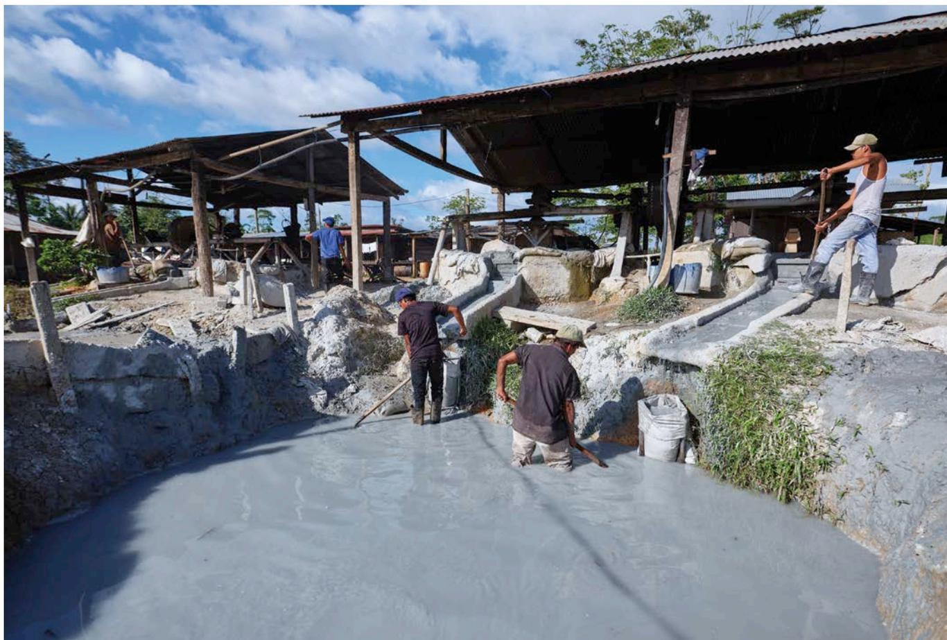
Water is an essential ingredient of artisanal processing, sourced from streams, circulated through the rastras (the preferred processing system used by the locals), and returned to the waterway. Copyright: Calibre Mining Corporation.
