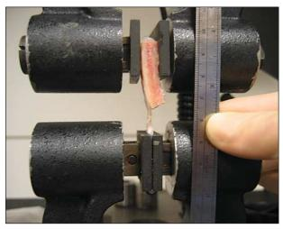
Figure 2. Bone and periosteum complex loaded into Instron Model 5500 (Instron Corporation, Norwood, Massachusetts).
