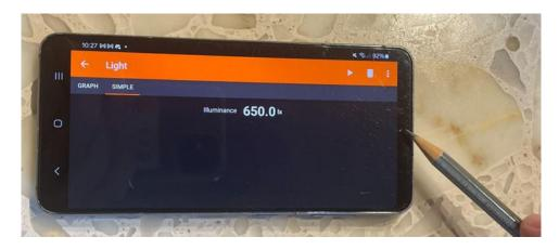
The pencil is pointing at the light sensor on this phone. It is helpful to rotate the display so the reading is clear of where the sensor will be held against the Pringles® tube.
