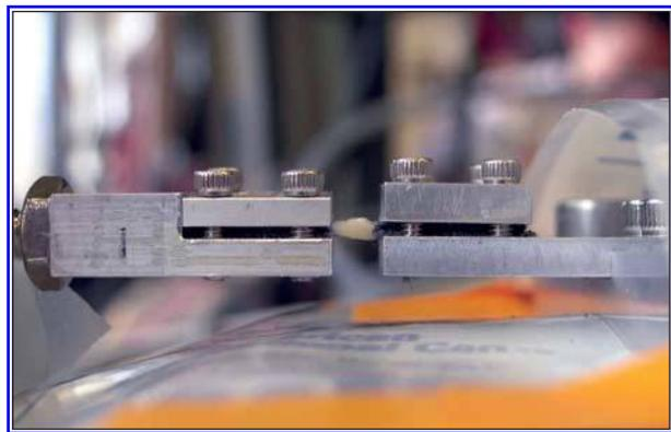
**Figure 2.** Testing device with cartilage sample in place. Samples were clamped sufficiently to avoid slippage while avoiding damage at the contact points at the end of the test gauge. The force transducer is shown on the left, and the motor is shown on the right.
