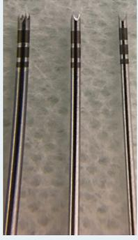
The sharp/blunt system in the original robot (released in 2011) used a 1.0mm sharp pronged needle that penetrated the skin about 1mm and was immediately followed by a rotating, dull punch with a slightly larger diameter that went deeper into the scalp. The current system includes a 0.9mm needle that is the workhorse for most cases. With refinements in the optical system, the needle/punch diameter was able to be reduced further. The new needle option is 0.8mm.
