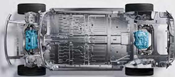
Front Double Wishbone + Independent Rear Five-link Suspension
