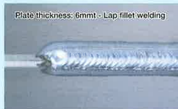
Welding current: 210A, Welding voltage: 23V Welding speed: 55cm/min, Welding wire: A5183, 1.6φmm
