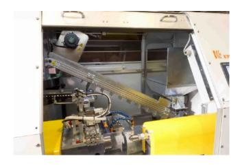
• Tip Conveyor Function Additional 800 tips can be supplied.
