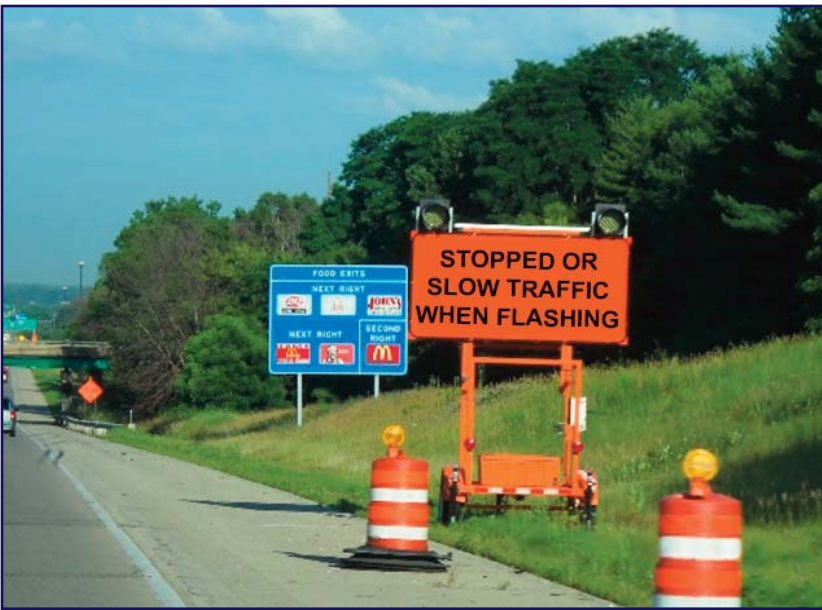
Figure 17. Stopped or slow traffic warning sign activated when queues are detected (Source: Illinois DOT).
