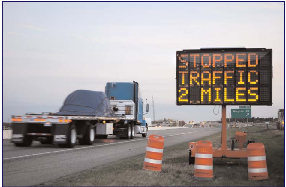
Figure 16. Message displayed on a queue warning system (Source: Texas A&M Transportation Institute).
