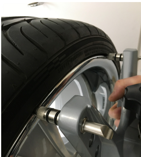
Gripper attachment on steel and aluminium rims
