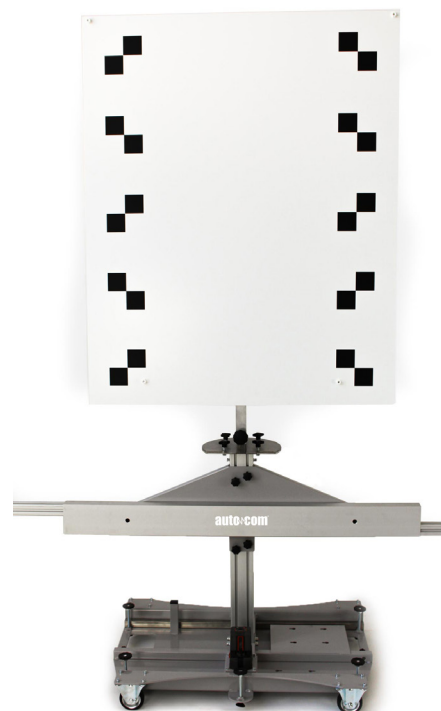
Lowest board position for calibration on buses.
