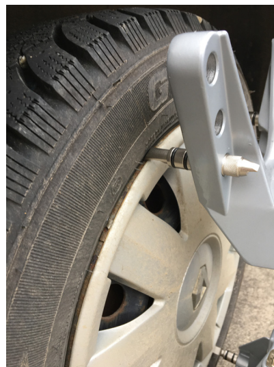
Long gripper side with mounted hubcaps
