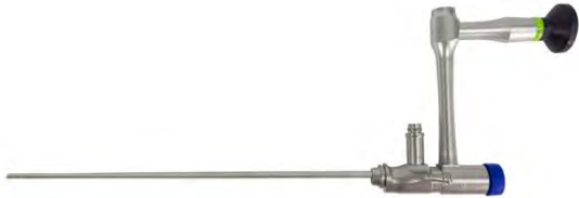
Nephroscope Parallel view Direction of view: 0° Working Channel: 15Fr. Ø Working Length: 250mm
