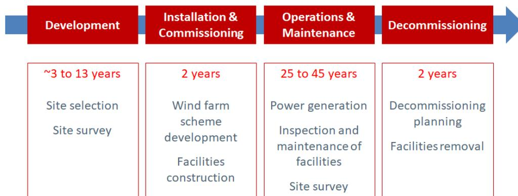
Figure 4.5: Indicative Offshore Wind Project Lifecycle Stages
