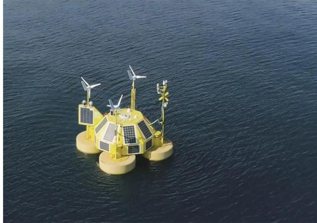
Figure 4.8: Typical Floating Lidar Buoy [15]
