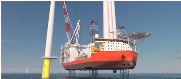
*Figure 4.10: Typical Jack-up Installation Vessel*
