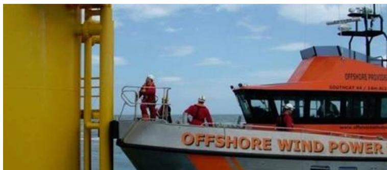
*Figure 4.13: Typical Crew Transfer Vessel*
