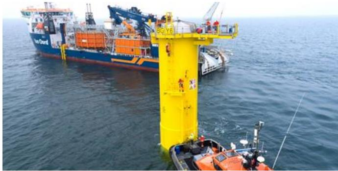
*Figure 4.9: Typical Cable Installation Vessel*
