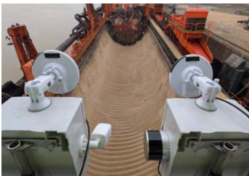
Two lidar devices installed on railings above the hopper of a dredger
