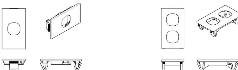
**product description** The straight data tile's have been designed to sit alongside the Lettric Face mounted Power Modules. It can be used for face mounting anything that fits into an Australian standard communications jack mount plate. e.g. switch mechanisms, neon's, USB connector etc. In-built clips allow it to mount into panels from 1.00 mm – 2.20 mm in thickness.
