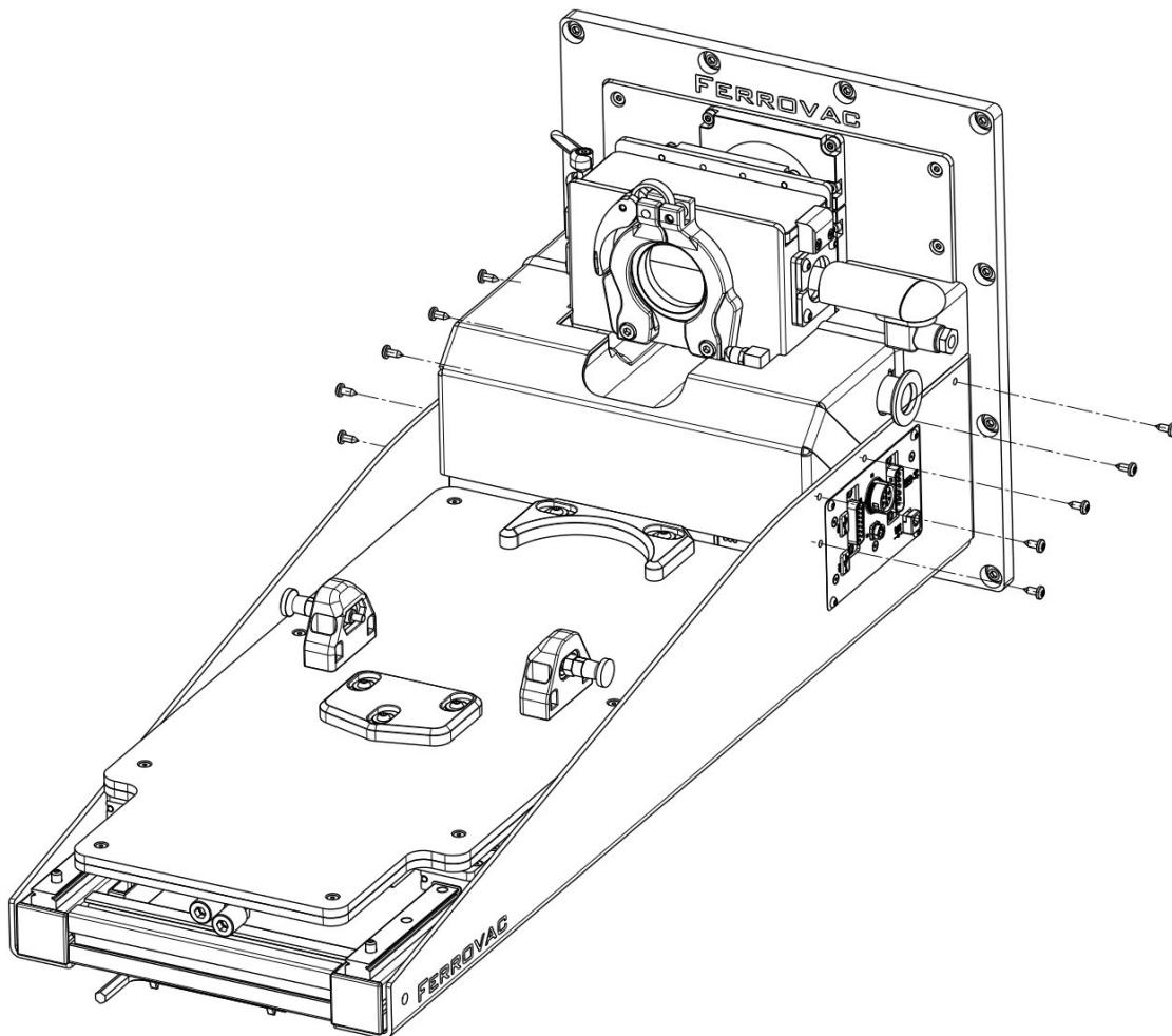
3. Remove the front part of the protective covering by carefully tilting it and moving it up- and outwards.
