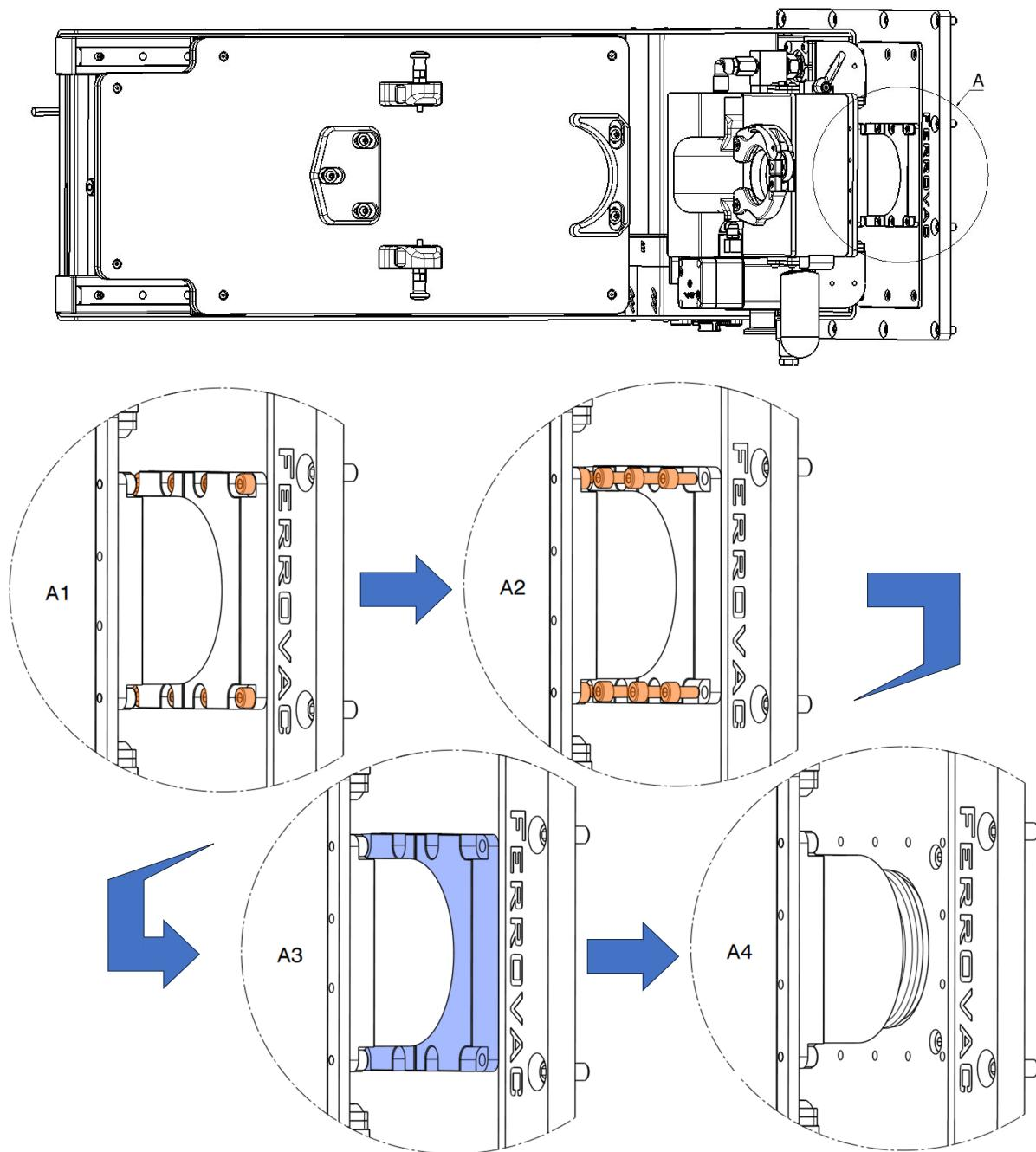
6. Once the gate valve is detached from the adapter plate (step 5), the pumping unit can be twisted slightly. This can help to remove the KF viton gasket between gate valve and adapter plate. It will also allow for better removal of the two plates mentioned in step 5.
