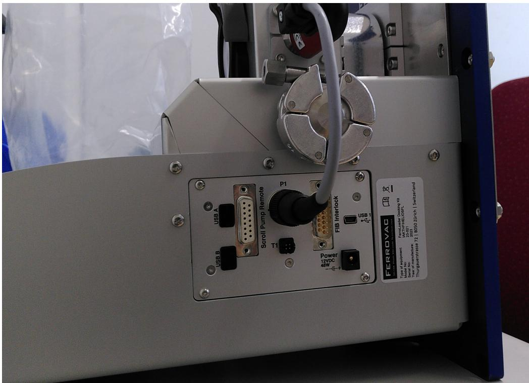
e) **If an Edwards nXDS Scroll Pump (103-190l/min, Ferrovac Product Code: PUS103 or PUS190) was part of the package:** Connect the roughing pump to the KF16 port using the appropriate roughing line and connect the D-Sub 17 connector between the electronics box and the Scroll pump with the D-Sub cable that is delivered with the package.
