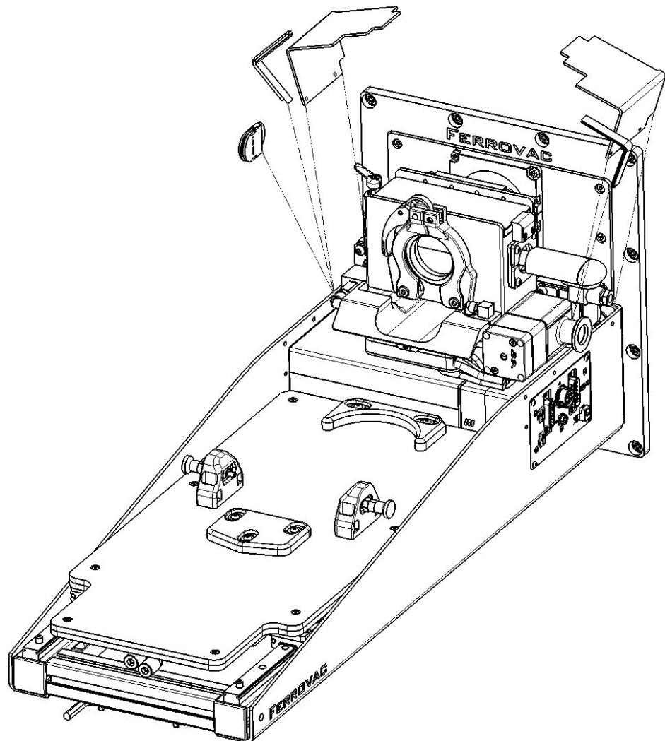
5. On the L-port frame of the dock, remove the 8 head socket screws and the two plates that hold the gate valve and the adapter plate together. Follow steps A1 to A4 to do so.
