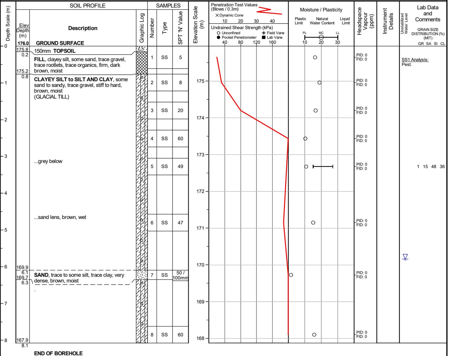
Unstabilized water level measured at 5.8 m below ground surface; borehole caved to 6.1 m below ground surface upon completion of drilling.
