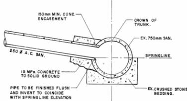
DETAIL OF 250 Ø A.C. SAN. CONNECTION TO EX. 750 Ø SAN. SEWER
