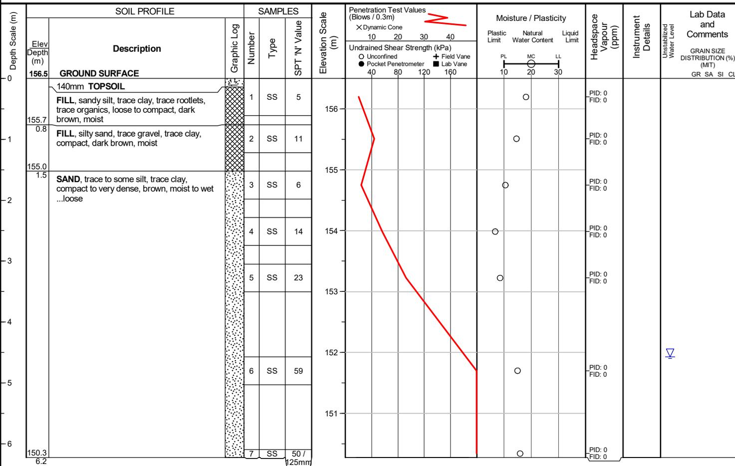
Unstabilized water level measured at 4.6 m below ground surface; borehole caved to 5.2 m below ground surface upon completion of drilling.
