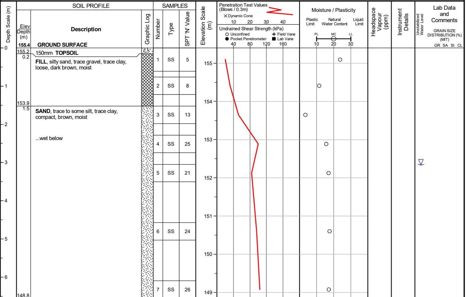
Unstabilized water level measured at 3.0 m below ground surface; borehole caved to 4.9 m below ground surface upon completion of drilling.
