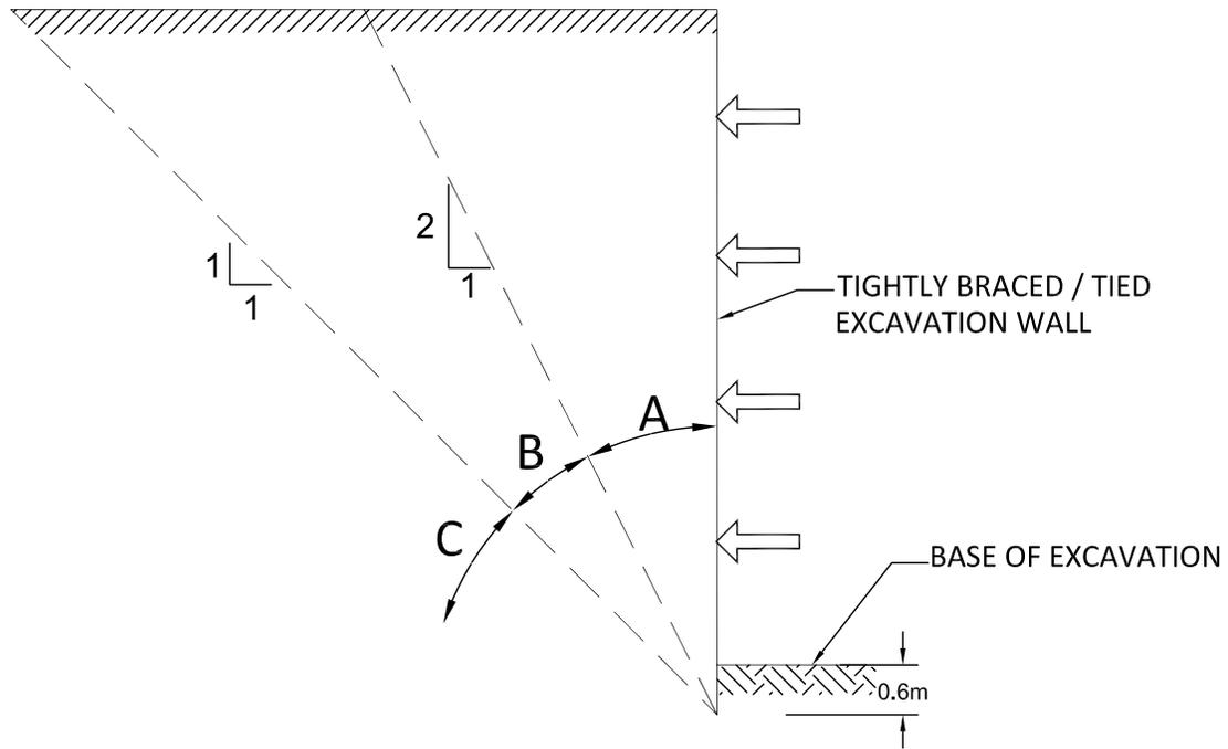
Zone A: Foundations within this zone often require underpinning. Horizontal and vertical pressures on excavation wall of non-underpinned foundations must be considered.
