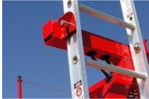
Photo 3, Portable aluminum ladder, retention studs engaged in storage slots.
