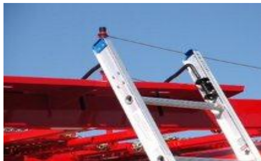
Photo 5, Ladder hooks engaged in slot behind catwalk.
