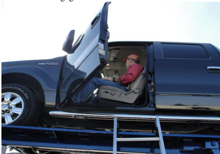
Photo 6, Ladder set up to access rear upper headramp position. Ladder hooks are engaged in slots in deck.
