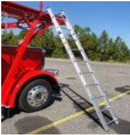
Photo 4, Portable aluminum ladder set up to access position over hood.
