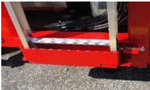
Photo 2, Bottom of portable aluminum ladder locked into place.
