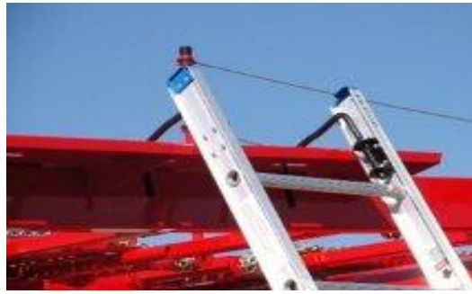
Photo 5, Ladder hooks engaged in slot behind catwalk.
