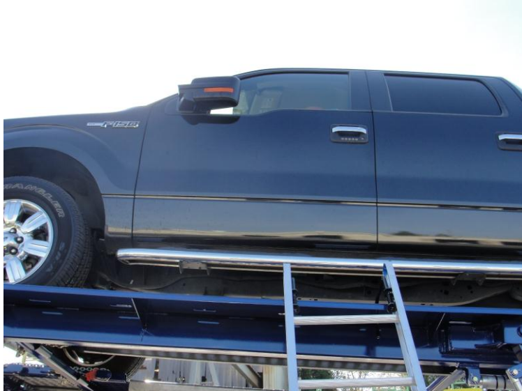
Photo 6, Ladder set up to access rear upper headramp position. Ladder hooks are engaged in slots in deck.
