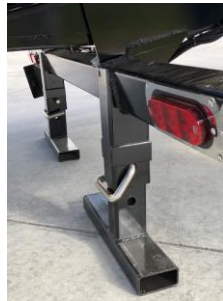
Photo: Both adjustable Stabilizing Legs must be firmly on the ground prior to loading or unloading, with locking pins in place.
