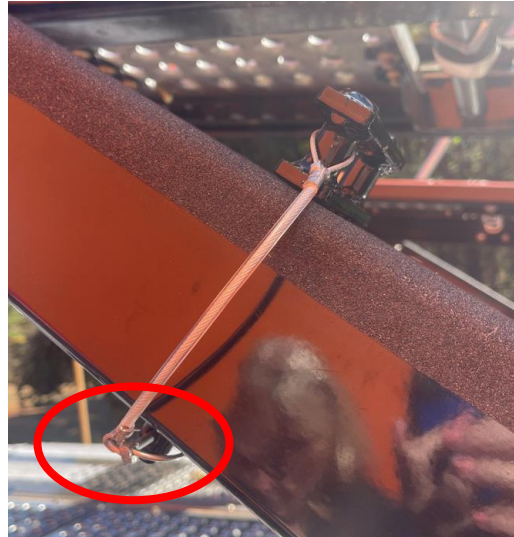
Deck Lock Pin secured with Linch Pin
