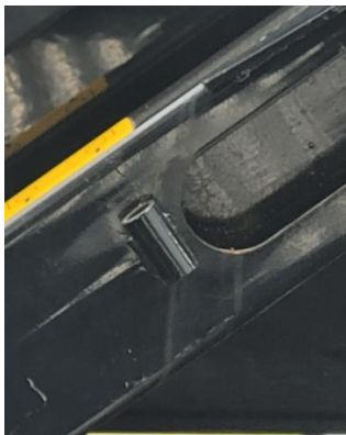
Deck Lock Pin Storage Location
