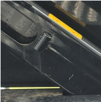
Deck Lock Pin Storage Location
