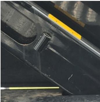
Deck Lock Pin Storage Location
