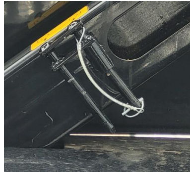
Deck Lock Pin secured with Linch Pin in storage location.
