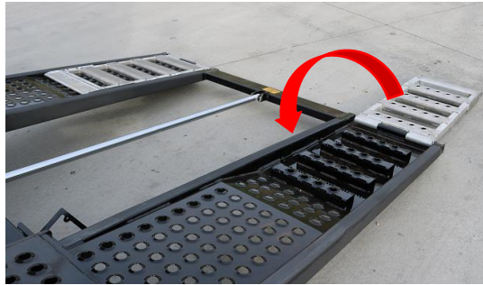
Flip Loading Ramp Extensions into Transport Position
