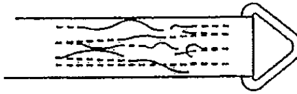
Figure 2 Broken Or Worn Stitching In Load Bearing Sew Patterns
