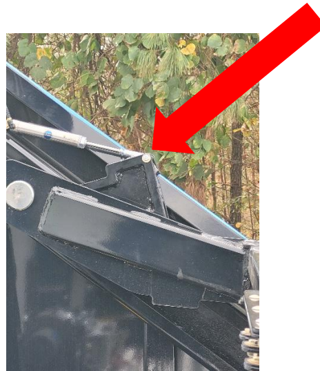
Deck Latch Disengaged
