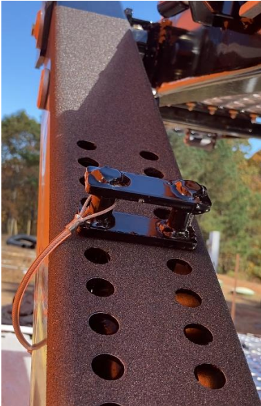
Deck Lock Pin Placement in Lowest Unblocked Holes on Lift Arm
