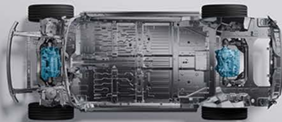
Front Double Wishbone + Independent Rear Five-link Suspension
