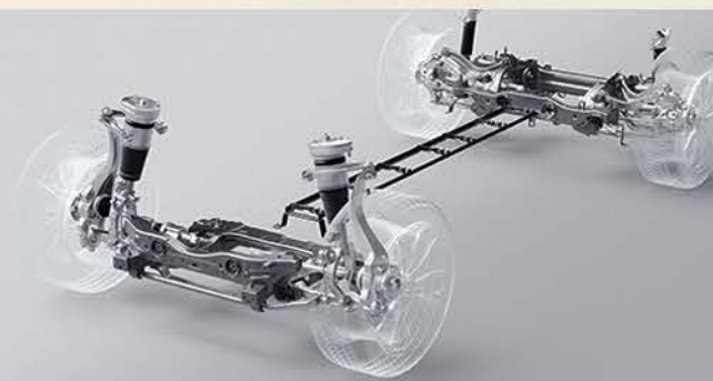
ZEEKR Magic Carpet Air Suspension with CCD
