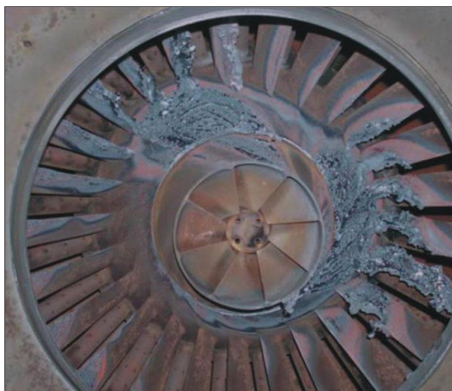
Figure 6.8 – Gas Turbine Damage by Flash-back. (Reproduced with permission of E.ON UK)
