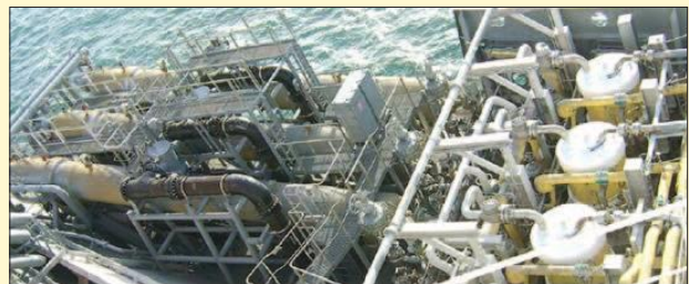
Figure 4.21 – Steam / seawater Vaporisers on Board the Excelsior .
