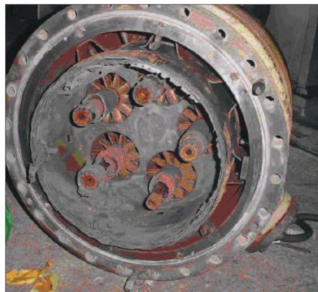
Figure 6.9 – Impact of Combustion Dynamics and Combustion Oscillations.
