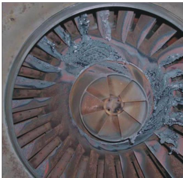
Figure 1.1 – Gas turbine – Damage from Flashback. (Reproduced with permission of E.ON)
