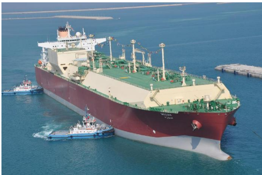
Figure 4: The Mozah Qmax LNG carrier at Ras Laffan. The Qmax fleet are the largest LNG carrier ever built, often modifications are required before a terminal can receive a vessel this large. Photo from wikimedia.org
