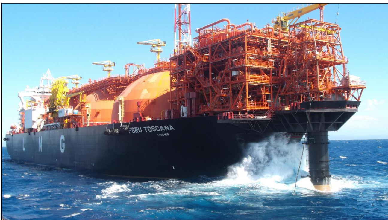
Figure 5: The FSRU Toscana located offshore Italy is a conversion of the LNG Carrier Golar Frost. Photo from https://commons.wikimedia.org
