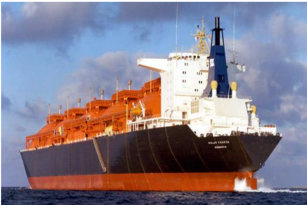
Figure 15: The Golar Freeze LNG Carrier, which was converted to serve as an FSRU in Dubai. Photo courtesy of Shell.
