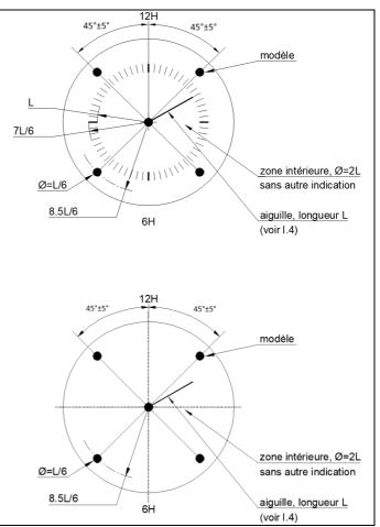
Dimensions in mm, general tolerances $\pm 200 \mu$  m, needle axis concentricity tolerance $\pm 400 m\mu$
